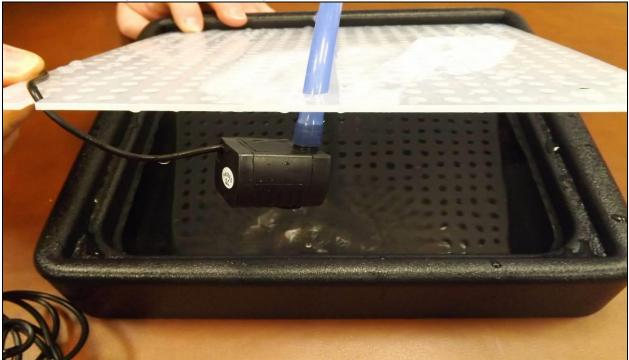
**Step 3:** Place the pad on the tray and align the vessel Luer fittings with the tube Luer fittings.
