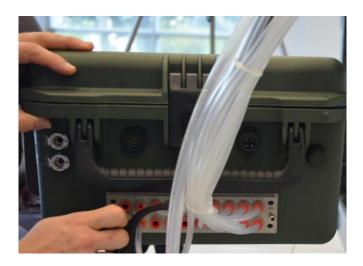
Connect the heart pump lines as shown, pump into-pump in and pump out-to-pump out on the control box side,
