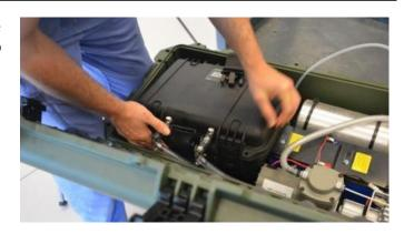
Place the Patient on the table upon its side ensuring the opening in the table is unobscured. Put the air control harness, the two heart tubes and the wire harness through the opening in the table.
