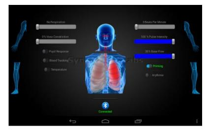
The pulse intensity is analogous to systolic pressure and base flow is analogous to diastolic pressure. These sliders may be operated independently to adjust the pulse pressure. By default, both sliders are at the maximum.
