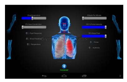
Selecting the Blood Tracking button will activate the physiology engine. This tracks and calculates the amount of "blood" lost and adjusts the heart rate, systolic, diastolic and pulse pressures, pupil response, vasoconstriction, thermal output and heart rhythm as the Patient losses "blood".
