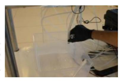
Once the water is clear, press the prime button again to stop the pump, connect the venous to the arterial fittings on the body to each other and the venous to the arterial fittings on the pump to each other. Press the prime button again to flush the venous side clear for 10 seconds. Turn off the control box and disconnect the sump, empty the sump and rinse it again. Ensure it is fully dry before returning to the control box.
