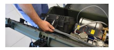
Use care not to damage the control board while the control box is open. Fill the sump with water or blood analog.
