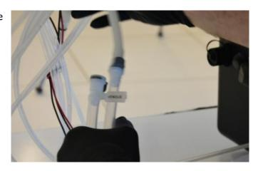
Plug the wire harness into the control box.
