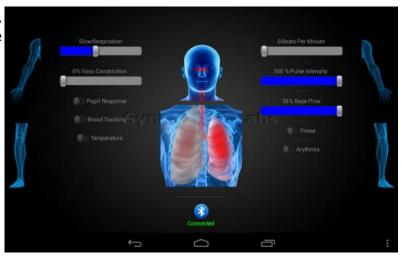
Each lung may be isolated to represent a collapsed lung by pressing on the lung icon you wish to deactivate. Once pressed, the icon will turn grey. Press again to restore function.
