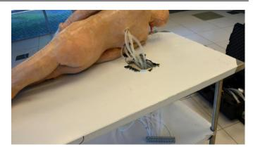
Place the closed control box under the table. Connect the air control harness to the front of the control box as shown and tighten the three Allen screws.
