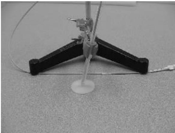
**Figure 2.** Holding Fixture.
