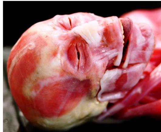
Individual models are constructed so that they mimic both the geometry (density, shape, length and diameter) and physical properties (water, salt and fibre content, modulus in tension, compression, and shear, coefficient of static or dynamic friction, surface energy, dielectric properties) of the portion of the human anatomy they are designed to match.
