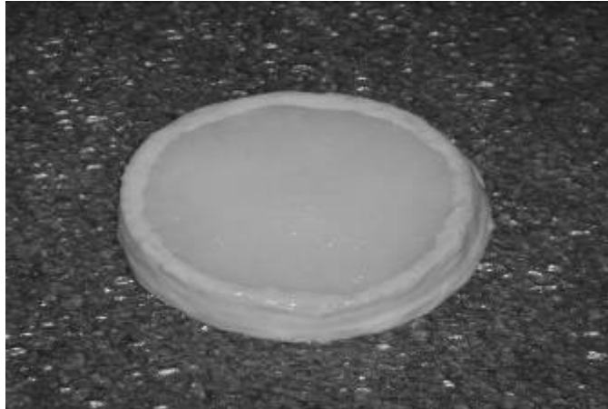
Figure 1. Arterial Tissue Disc. This multilayer tissue disc includes synthetic muscle, fascia, fat, and arterial intima.
